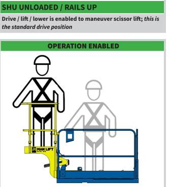
Drive / lift / lower is enabled to allow maneuverability into working position
