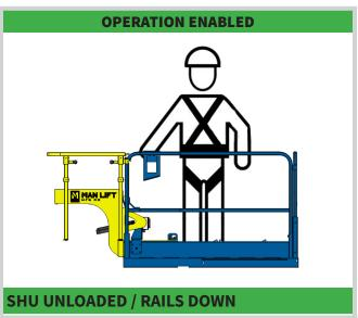
Drive / lift / lower is enabled to maneuver stowed SHU through narrow areas such as doorways
